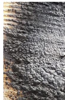
Intumescent Fire protection of WOOD FR-BAR.45
